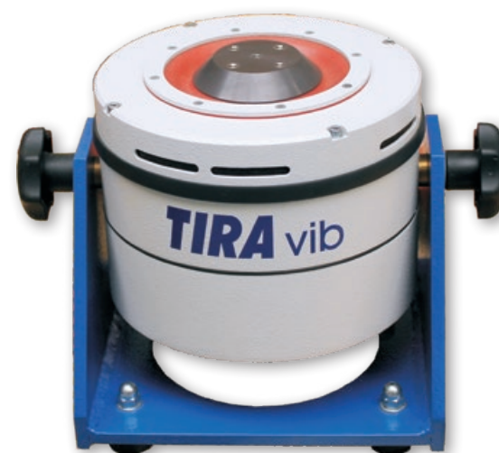
Calibration Shaker S 51140-C
