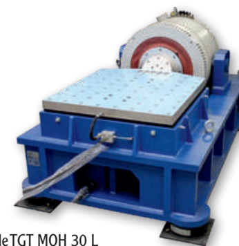
Shaker S 57315/LS-340 with slip table TGT MOH 30 L
